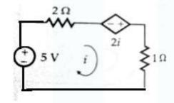
2 a) Find the power loss in 1  $\Omega$  resistor by Thevinin's theorem
